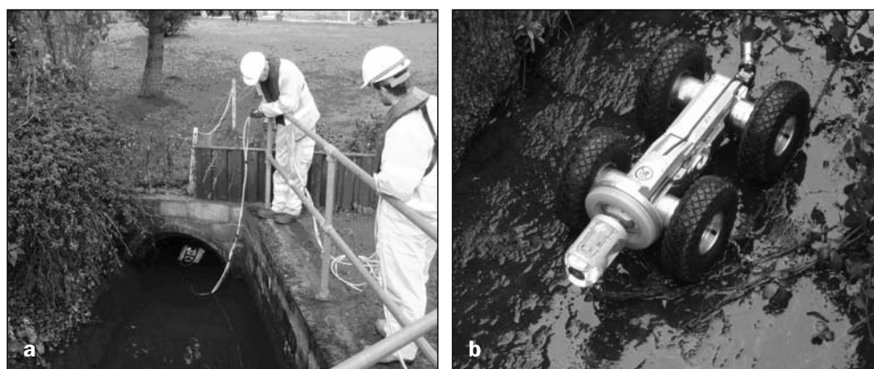
Figure 7.2 Culvert inspection using a CCTV system (a) and a typical tractor unit and CCTV camera (b) (courtesy Environment Agency and British Waterways)
